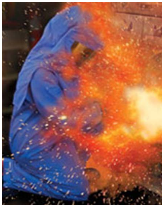
Figure 1: An electrical arc flash delivers an extreme heat and pressure wave with deadly force.
